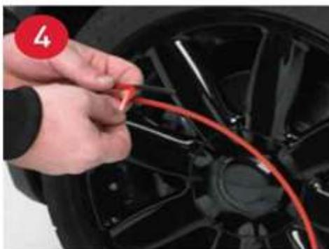
5. Carefully peel off backing from the tape in small sections at a time whilst applying to the wheel. Do not handle the sticky surface of the tape as this could potentially reduce the adhesion.
